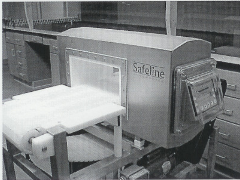
Figure 1. Safeline, Inc Power Phase metal detector used to conduct needle detection testing.
